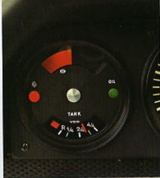
The combi-instrument for the temperature, fuel gauge and oil warning light also displays the warning light that tells you the handbrake is on.
